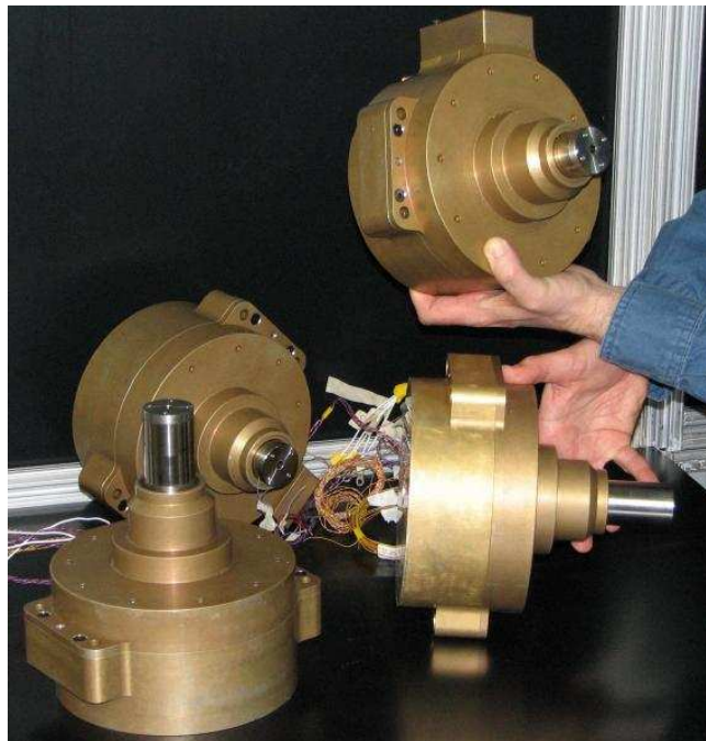
Figure 6. Serially Connected Three-Slice Linear Actuators
