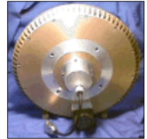
Custom 14" hub-style TENV motor built to power a solar race car ( http://www.e-torq.com )
